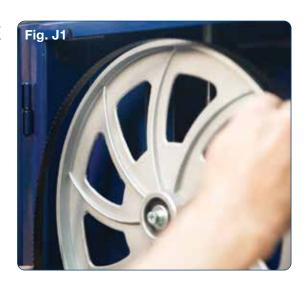
Replacing the blade is simply the same procedure in reverse, understanding that the bearing guides may need adjustment to accommodate the new blade. Remember to re-lock everything and adjust your tension and guides systems before use!
